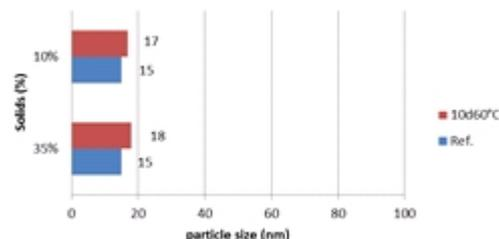
Particle size stability of UCECOAT® 2805 when submitted to accelerated ageing tests at 60°C in normal and diluted form
